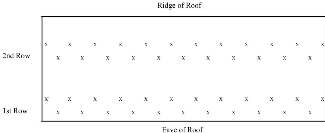
*Above example is based on Metal Roof Panels being 36" Panels with 9" rib spacing.*
